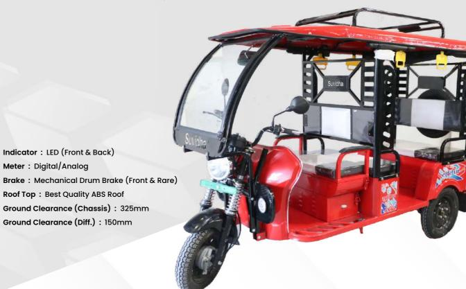
Rim: Metaliic/Alloy Tyre Size: 90\*90\*12 Controller: 24 Tube Differential: 33-42 inch Head Light: Rajulex
